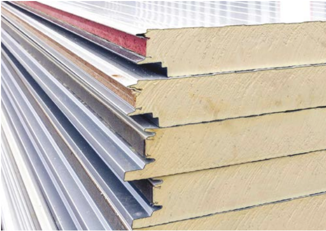
Figure 13. Left: Insulated metal panels (IMPs) are fabricated by blowing polyisocyanurate foam into aluminum skins in a continuous, high-volume automated process. Photograph courtesy of by DJ Srki.
