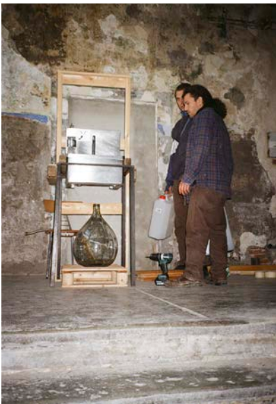
Figure 7. Cucina (kitchen) team testing a sink with water recycle system, aiming for sustainable and autonomous forms of cohabitation. Photograph by Yona Catrina Schreyer.
