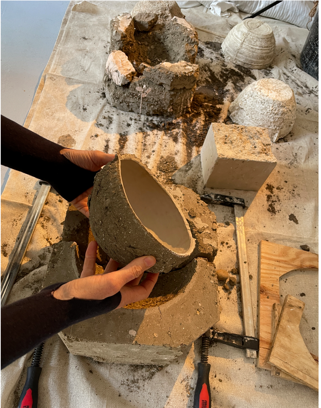
Figure 7. Handling a drying slip cast bowl.
